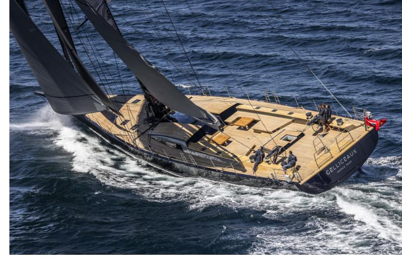
"The production of SW108 begins with a well-canvassed, very powerful arrangement for exceptional performance in light winds, but also up through the wind range. SW108#01 owners were keen on the hybrid propulsion system which adds weight and some propeller installation drag.
