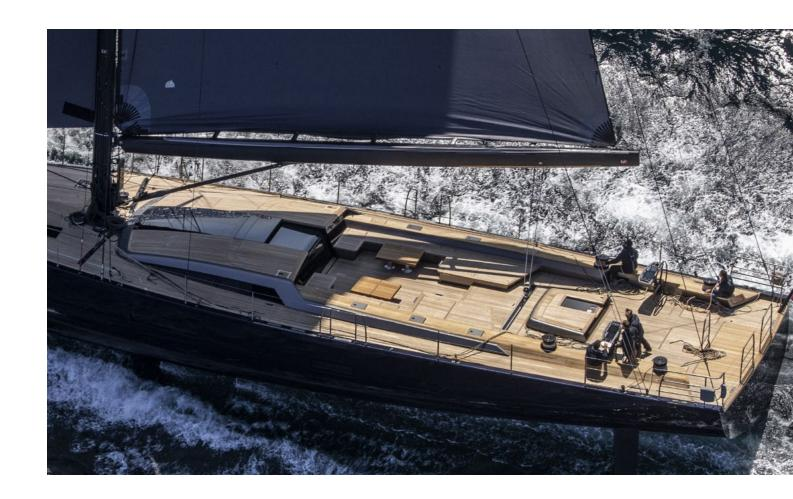
"Gelliceaux deck layout is fresh but immediately recognizable for its clean, sober geometries that include all the touchstones of the GT look in a new configuration. SW108#01 has a coachroof that allows lots of light to flow into the yacht through a central skylight and side windows.
